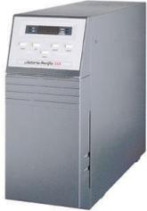
The optional 315 UV/Vis detector uses either a deuterium lamp or tungsten lamp to measure UV or Visible wavelengths respectively. This detector is a good choice for Breweries monitoring Bitterness (in UV configuration plugged into an Astoria or Astoria2) or labs monitoring vitamins in Fortified Flour Extracts (i.e. two fluorometers and one 315 visible detector running through a 350D A/D Module).
