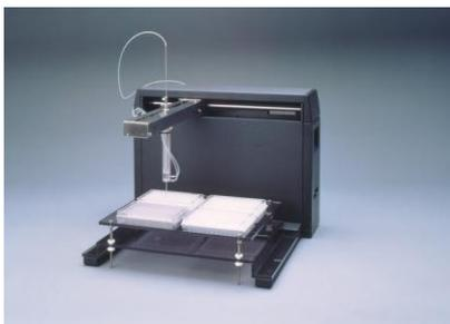
The 311 is a versatile random access sampler. Many of its features include: a Travelling Wash Pot that ensures consistent inter-sample bubbles between samples and wash; a separate standards/calibrant rack that reduces time spent on pouring standards; the use of different sizes of sample cups and sample racks; use with an optional diluter that can automatically dilute off-scale samples and allow the user to create standards/calibrants online.
