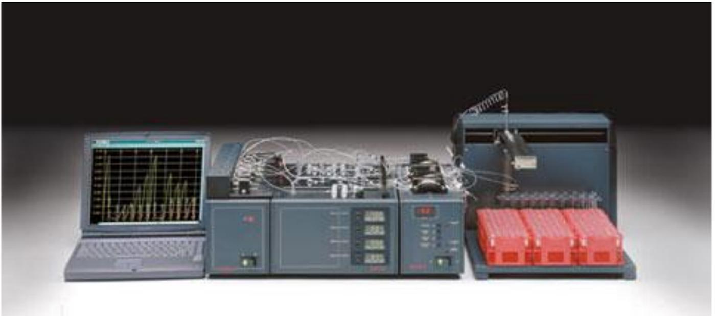
This is the flag ship model of Astoria-Pacific's Industrial Division. The system's six-channel digital detector is ideal for laboratories (i.e. Oceanography, Tobacco, etc.) that want to test four to six parameters from a single sample. Using micro-Segmented Flow Analysis, the Astoria Analyzer follows the modular design layout (pictured above):
